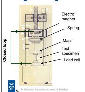
The oscillator (spring – mass system needs small I/P effect (current to the electro magnet) to maintain a sinusoidal motion at its resonance frequency
