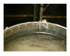
By using several strain gauges stress gradients can be measured
